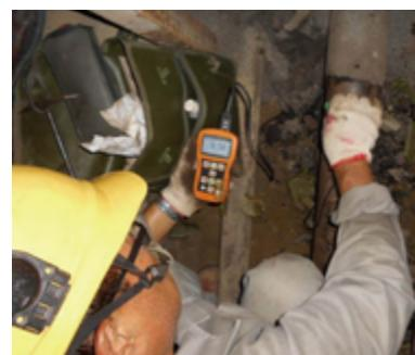
Soil and pipeline thickness analysis
