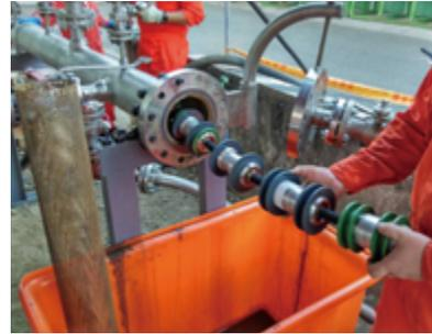
Pipeline intelligent inspection instrument
